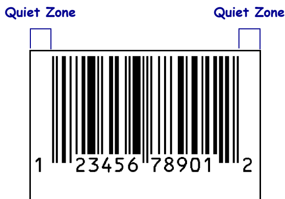
Figure 9 • Quiet Zone in a Bar Code
