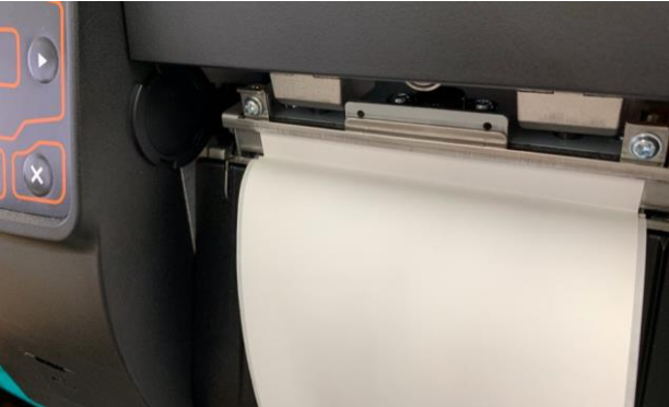
label stuck to the ribbon guide
