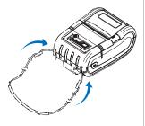
Insert the strap into the hook on the printer.
