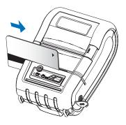
Insert and swipe the card in the direction of the arrow as shown in the picture.
