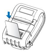
Insert the card in the direction of the arrow as shown in the picture.
